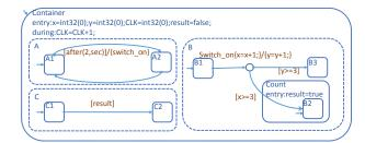
Fig. 2. A Stateflow example for counter task which covers most advanced modeling features.
