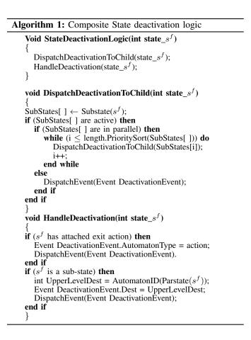
After the execution of *controller automata* on the logic of state active or deactivate, *action automata* will continually read the stack top event for the test of the guard. The guard on the three transitions are StackTop().Event == ActivationEvent, StackTop().Event == DuringEvent and StackTop().Event == DeactivationEvent. Then, the transition with satisfied guard will take, and corresponding action statements in Stateflow are translated to action statements attached on the three transitions.
