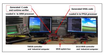
Fig. 8. Real system platform simulation between D113 controller and TiMVB controller. The left is the implemented TiMVB, and the right is D113.
