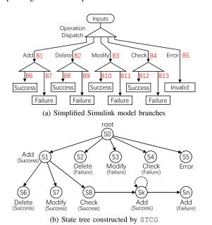
Fig. 3. An example of STCG corresponding to the model in Figure 1. (a) shows the simplified model branches, which contain a total of 13 branches. (b) illustrates the state tree with the full coverage explored.
