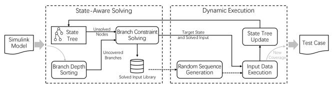
Fig. 2. Overview of STCG. Two parts are executed cyclically to obtain test cases. The State-Aware Solving part focuses on obtaining the one-step input data by constraint solving on one iteration of the model. The Dynamic Execution part focuses on obtaining the specific state of the model by executing the solved input data and outputting test cases.
