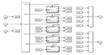
Fig. 1. An example of model with complex internal states. This is an AutoSAR CPU task dispatch model. It mainly contains the four operations of adding, deleting, modifying and checking CPU task in the queue.
